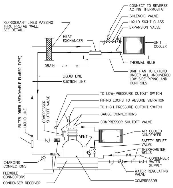
REFRIGERANT PIPING DIAGRAM FOR (INDOOR FLOOR MOUNTED COMPRESSOR)
